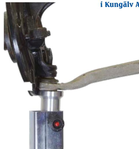
The upper frame can be mounted upside-down and be used as a lifting jack when working with other jobs on the suspension system.
